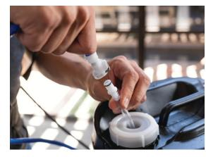
STEP 2: Insert the quick-connect devices into each other, found on the 30' blue hose and the tube attached to the 5-gallon container cap.
