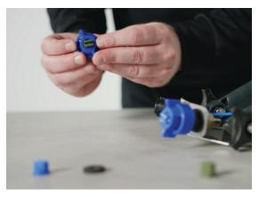
STEP 2: Push spray tip out of lock nozzle cap and replace with desired spray tips. Place sprayer tips in first, followed by the rubber washer.
