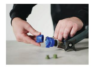
**STEP 1:** Twist lock nozzle cap counterclockwise. Handle with care, so as not to misplace spray tip and rubber washer.
